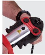
Connect with clamping jaws 8 mm
