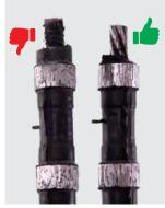
Remove residues from the substrate wire
