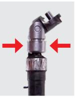
Make sure that the position of the clamping jaws is correct (see red arrows in the image)
