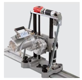
WM90 Saw head with PowerGear drive / Specifically suitable for wall saw blades bigger
