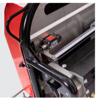
End switch for wire storage/ When the wire storage is full, the system is deactivated automatically (auto stop)
