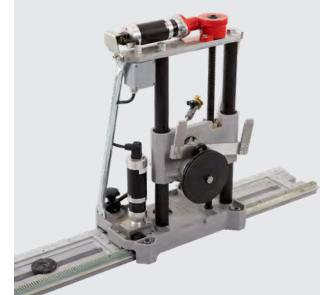
WM90 Saw head / Main bearing easily accessible from the blade flange
